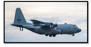
The EC-130H Compass Call is an airborne communications jamming platform. The EC-130 Compass Call aircraft attempts to disrupt enemy command and control communications and limits adversary coordination essential for enemy force management. The Compass Call system employs offensive counter information and electronic attack
