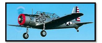
The BT-13 Valiant was an American World War II-era aircraft used for the United States Army Air Corps. It required the student pilot to use two-way radio communications with the ground to operate landing flaps and a twoposition controllable pitch Propeller. The flaps were operated by a crank-and-cable system.
