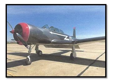
Chuji Jiaolian-6 abbreviated CJ-6 is a two-seat basic trainer and light attack aircraft designed and manufactured in China for the People's Liberation Army Air Force. The CJ-6 can be fitted with two 7.62mm machine guns, bombs, weapons stations and rocket launchers for light attack capability.
