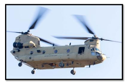
The win-engine, tandem rotor Chinook helicopter had undergone numerous upgrades since the first CH-47A model was delivered to the Army for use in Vietnam. The Chinook's cockpit accommodates two pilots and an observer. Three machine guns can be mounted on the helicopter, two in the crew door on the starboard side and one window-mounted on the port side.
