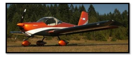
The RV-12 is equipped with a ground-adjustable Sensenich composite propeller — light, smooth and affordable. The light empty weight allows a generous and truly useful load — two 185lb people, a full tank holding 20 gallons of fuel, plus 50lbs of baggage. And it gets even better when
