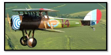
The Nieuport 28 C.1 is a French biplane fighter aircraft flown during World War I. The Nieuport 28 design advanced the concept of the lightly built, highly maneuverable rotary engined fighter. A shortage in 1918 led to Nieuport 28s being issued to four American squadrons, becoming the first aircraft to see operational service with an American fighter
