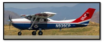
The Cessna 182T Skylane is a four-seat, single-engine, all-metal light airplane. The 182T has fixed landing gear and is powered by a fuelinjected 230-horsepower Lycoming IO-540-AB1A5 piston engine. It is the only variant in production. Civil Air
