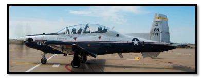
The T-6A Texan II is a singleengine, two-seat primary trainer designed to train Joint Primary Pilot Training Students in basic flying skills common to U.S. Air Force and Navy pilots. Steppedtandem seating in the single cockpit places one crew member
